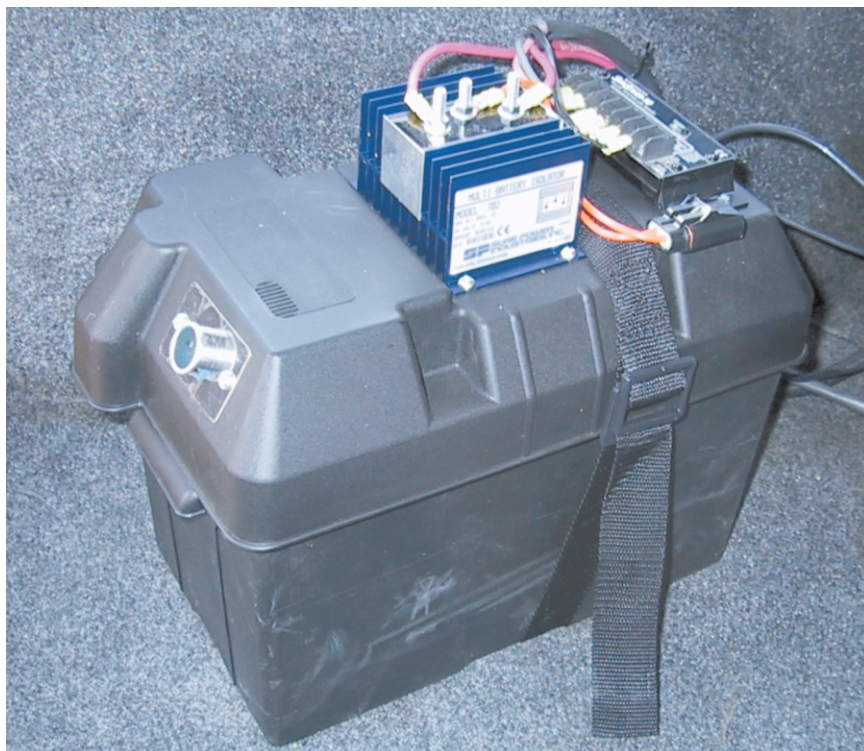
Completed battery box with top mounted battery isolator and solar charge controller
