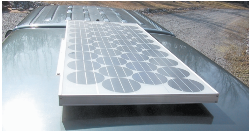
100 watt solar module mounted on roof of truck bed cap
